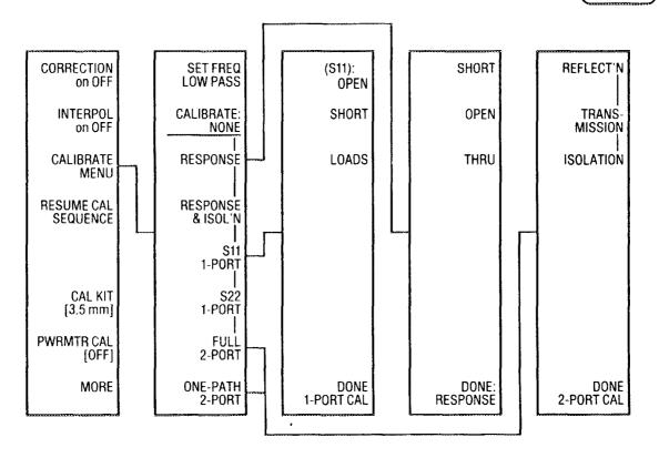
SET FREQ Changes the frequency sweep to accommodate time domain low pass mode (option 010). If this mode is used, the frequencies must be set before calibration.
