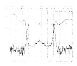
**DUAL CHAN** Displays both channels at once. They will be placed on separate on OFF graticules if split display mode (page 19) is on.
