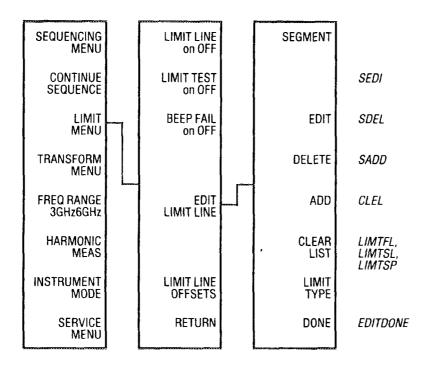
SEGMENT Selects the segment to be edited either by entering the segment number, or by using the front panel knob or step keys.
