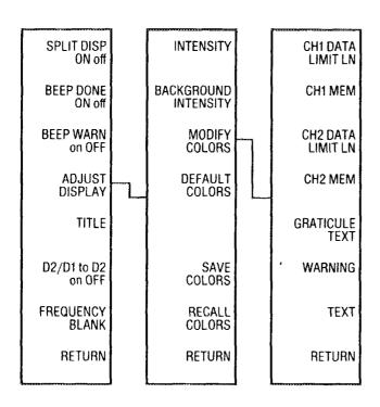
Note: these keys (except return) lead to a second color menu that allows modification of tint, brightness, and color. If varying tint has no visible effect, increase the color percentage first.
