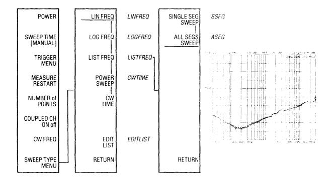
LIN FREQ Activates a simple linear frequency sweep. With option 010, the analyzer can translate this data to time domain.
