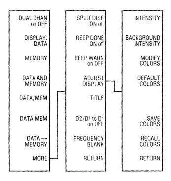
**INTENSITY** Sets the CRT intensity as a percentage of the brightest setting.
