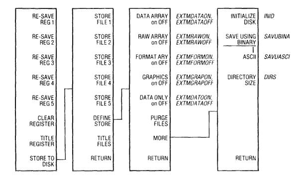
The disk access functions are controlled through the [STORE TO DISK] and [LOAD FROM DISK] menus under the [SAVE] and [RECALL] keys, respectively. In addition to the complete instrument state, some information that is not included in the internal registers can be stored on disk.
