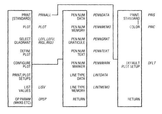
\*\*PRINT Copies the HP 8753 display onto an external printer. Identifies the printer selected; [STANDARD] (for black and white), or [COLOR]. The HP 8753 must be in either system controller or pass control mode.
